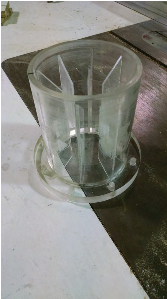
Figure 2: Vanes were installed in the pool between the FSI's and the pumps.
