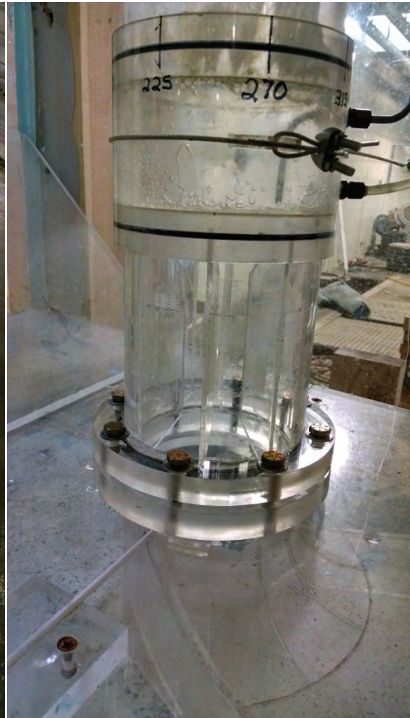
Figure 2: Vanes were installed in the pool between the FSI's and the pumps.
