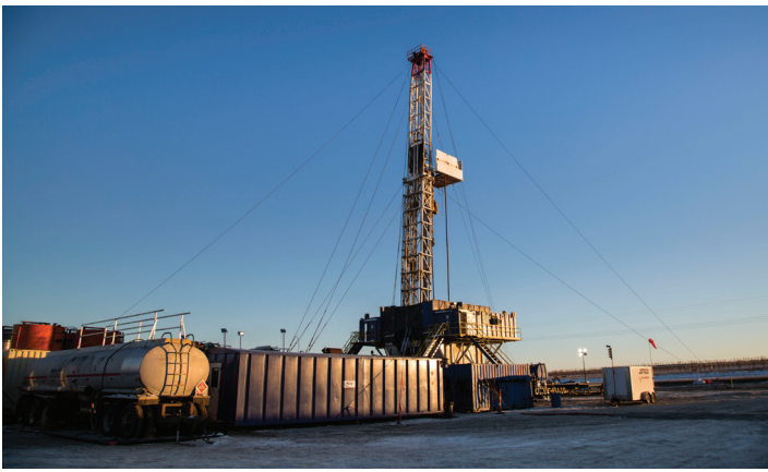
A drilling rig equipped to drill a test hole more than 2 miles deep to collect rock core and fluids as well as data about the rock layers, their fluids, and their pressures.
