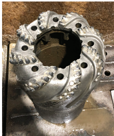
Multiple cylindrical rock samples called cores will be retrieved from a section of the hole using a specialized coring drill bit.
