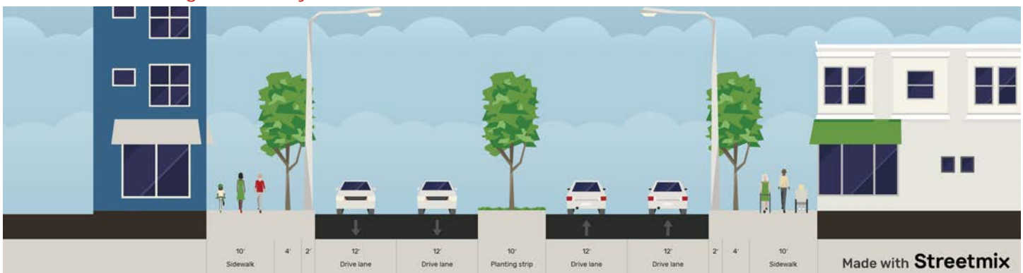
Figure 52 – Bicycle and Pedestrian Facilities on Four-Lane Commercial Arterials
