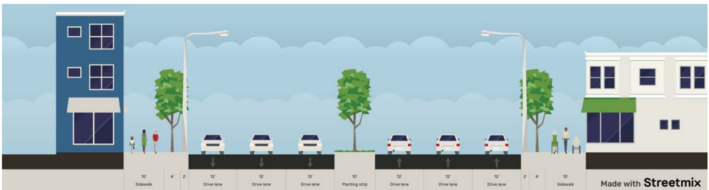
Figure 53 – Bicycle and Pedestrian Facilities on Six-Lane Commercial Arterials
