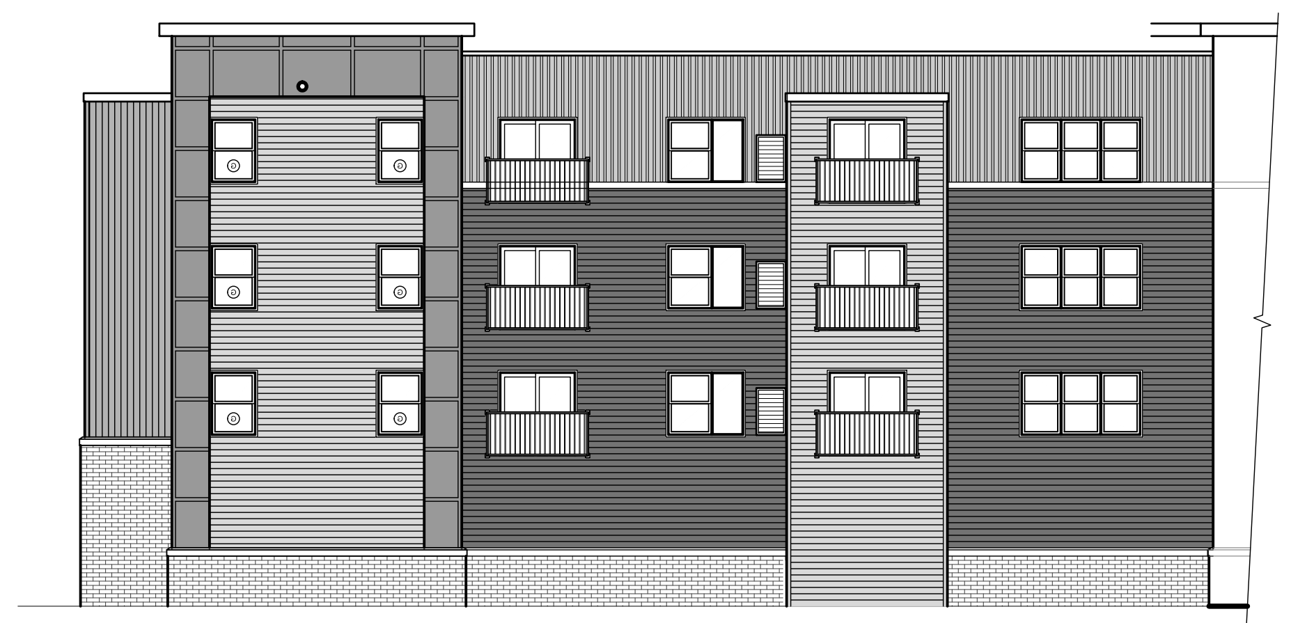
SOUTHWEST ELEVATION SCALE: 3/32" = 1'-0"
