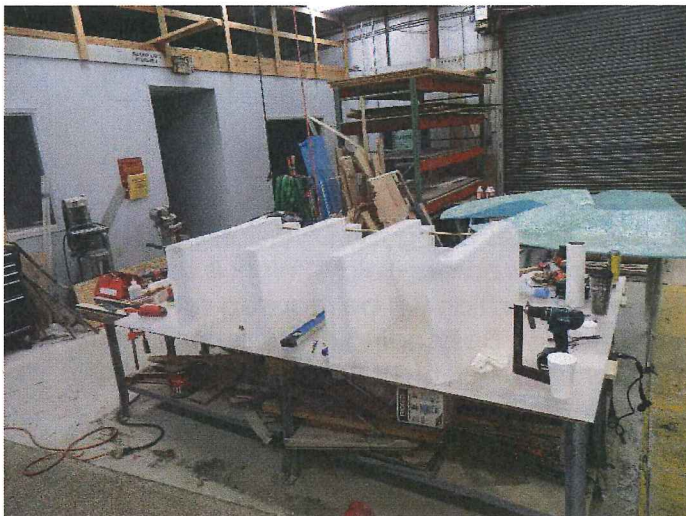
Construction of Red River physical model at ERDC
