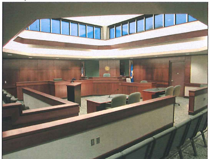
The courtroom features clerestory windows to provide ample natural light, while still maintaining privacy and safety.
